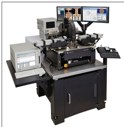
▲ Fig. 1 Typical WMS configuration with Keysight measurement instruments and Cascade Microtech probe station.
