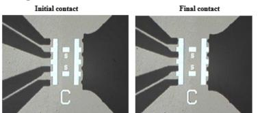
Figure 2: Images showing correct alignment and placement of probe tips of both ACP and Infinity style probes.
