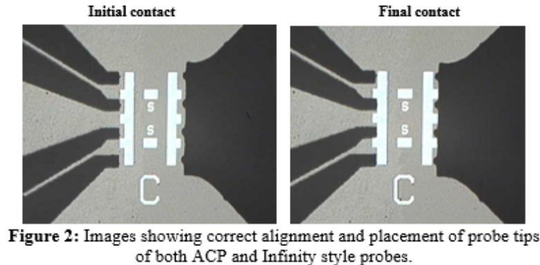
**Calibration Coefficients** are dependent on the probe tip configuration, placement on a standard, and the standard configurations. This leads to unique calibration coefficients for a unique pair of probe and ISS. Therefore, the calibration coefficients are supplied with the probe not with the ISS.
