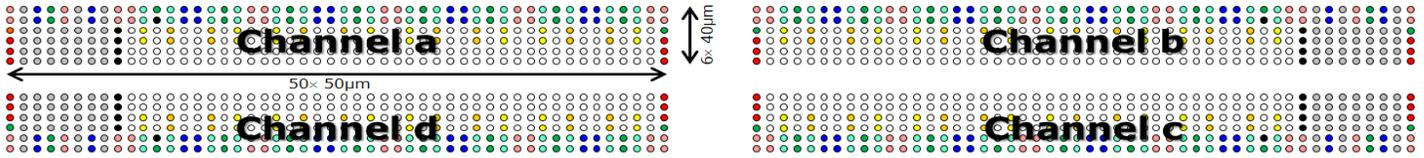
Figure 4: Standardized micro-bump lay-out according to the JEDEC Wide-I/O Mobile DRAM specification [19].
