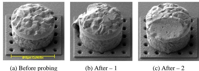
**Figure 17:** Probe marks on non-reflowed  $15\mu\text{m}$ -diameter Cu/Ni/Sn top micro-bumps.
