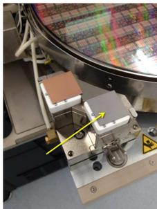
**Figure 15:** Tungsten-carbide (WC) tip cleaning substrate on CM300's auxiliary chuck.
