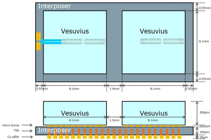
**Figure 11:** Vesuvius-2.5D test vehicle top view and cross-section.
