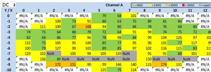
**Figure 20:** Wafer map with two-point resistance measurement values for DC 2 of Channel  $a$  on an Interposer wafer with Cu micro-bumps.
