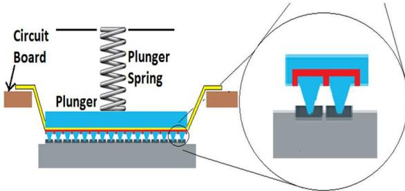
Figure 7: Conceptual cross-section view of the probe core [18].
