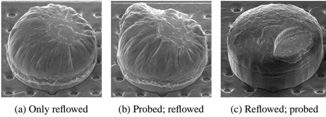
**Figure 18:** Probe marks on reflowed  $15\mu\text{m}$ -diameter Cu/Ni/Sn top micro-bumps.
