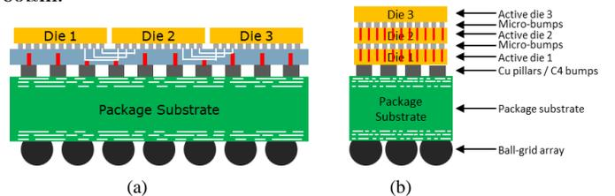
**Figure 3:** Cross-sections of typical (a) 2.5D- and (b) 3D-SICs containing three active dies.
