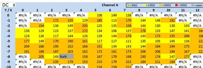
**Figure 21:** Wafer map with two-point resistance measurement values for DC 2 of Channel  $a$  on an Interposer wafer with Cu micro-bumps with a NiB cap.
