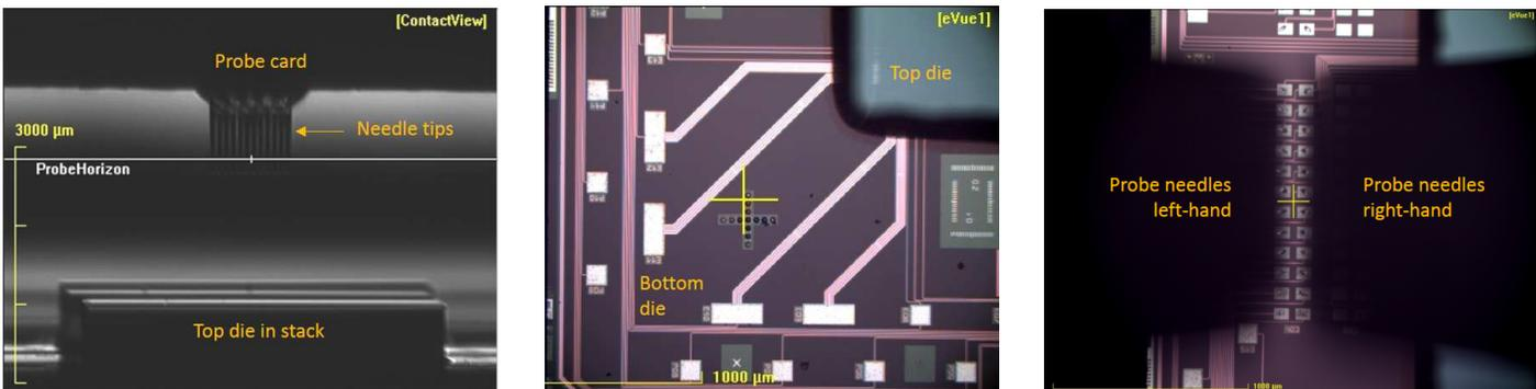
(a) Probe needles and die stacks; contact view from side-view camera.
