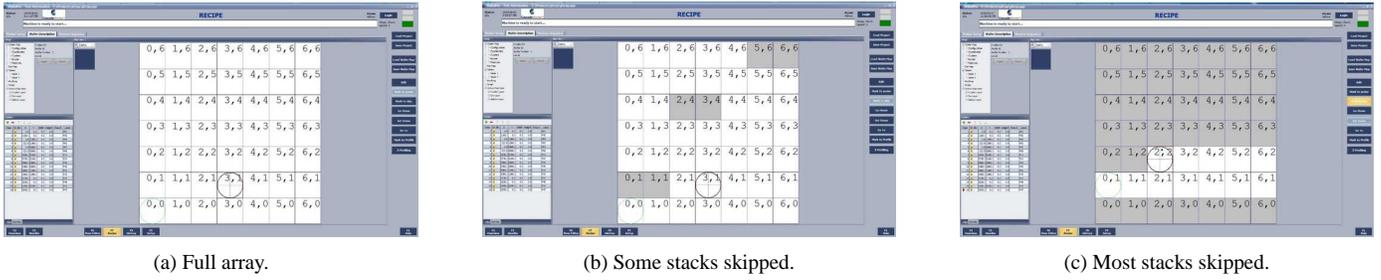
Figure 6: Example rectangular wafer maps for  $7 \times 7$  array of PnP'd die stacks.
