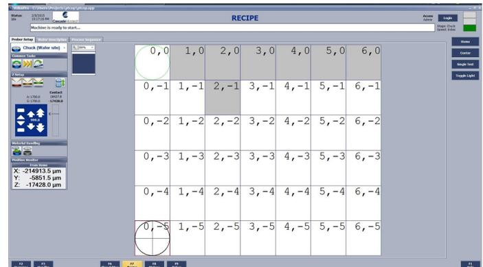
**Figure 18:** Wafer map of an array of  $7 \times 6 - 7 = 35$  PnP'd PTCO/P stacks on double-sided thermal-release tape.
