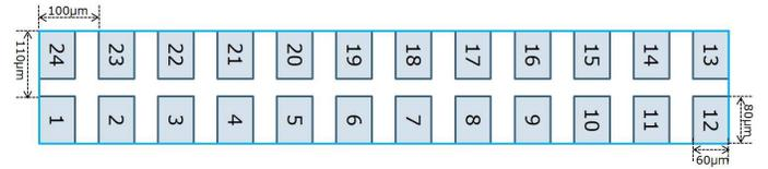
Figure 9: IMEC-standard  $2 \times 12$  probe-pad module.
