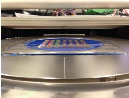
Figure 12: Used tape frame with slight bend.
