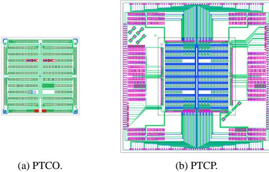
Figure 7: Layouts of 3D test chips (a) PTCO and (b) PTCP.
