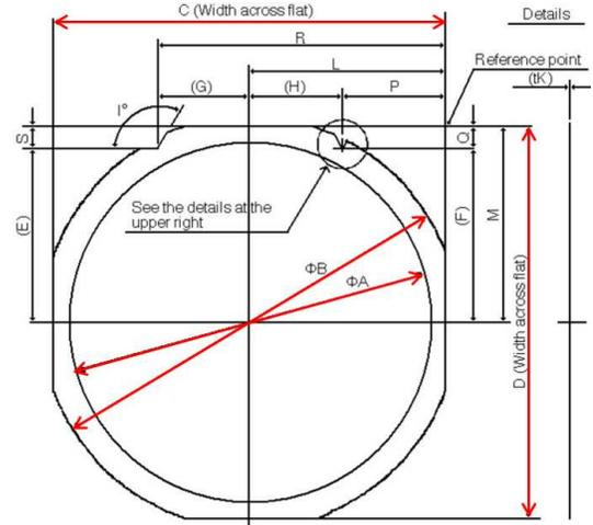
**Figure 19:** Specification of SEMI G74-0669 tape frame for  $\varnothing 300\text{mm}$  wafers (source: SEMI, [8]).
