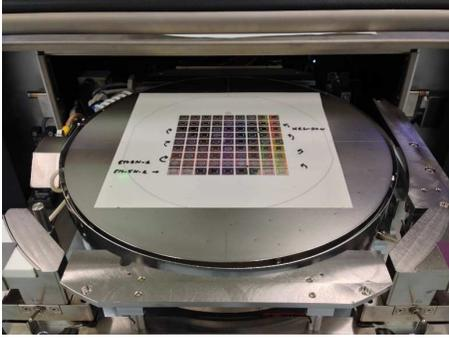
**Figure 15:** Loading a tape sheet with PnP'd die stacks onto the CM300's chuck via the prober's front-side manual load port.
