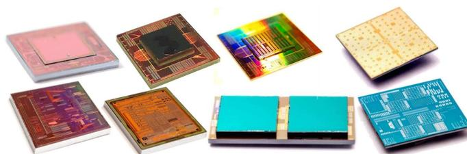
Figure 1: Examples of D2D-stacked 2.5D- and 3D-SIC test chips at IMEC.
