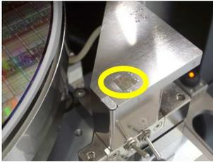
**Figure 3:** Manually placed D2D stack on the auxiliary chuck of a CM300 probe station.
