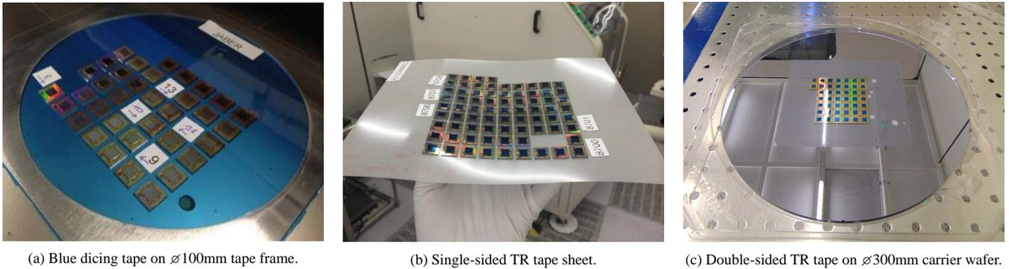
**Figure 10:** Three carriers with arrays of PnP'd PTCO/P D2D stacks.
