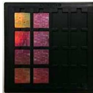
Figure 2: Example waffle pack, here holding eight singulated dies.
