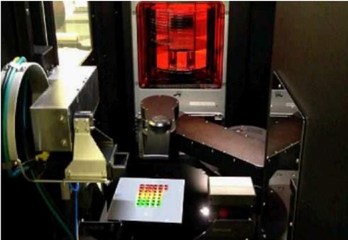
**Figure 17:** Carrier wafer with a sheet with PnP'd die stacks in the MHU.
