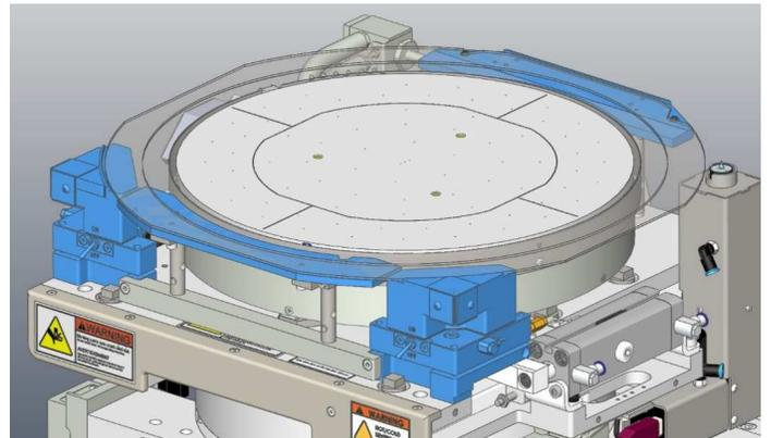
**Figure 20:** CM300 tape-frame support for SEMI G74-0669 [8].
