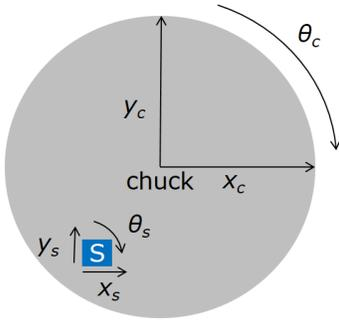
**Figure 5:** Translation and rotation misalignments and corresponding chuck compensation.
