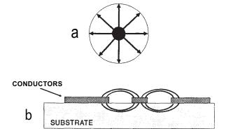
*Figure 3. Electric field patterns in coaxial and coplanar transmission lines.*
