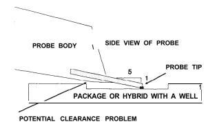
Figure 39. Side view of probe and package with a well, illustrating potential clearance problem.
