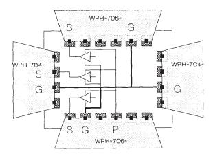
*Figure 15. Rule 201 - All probes must have at least one ground. Rule 202-All probe grounds must be connected together on the DUT.*
