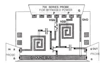
*Figure 26. Schematic of lumped-element MMIC. WPH-700 multicontact probe provides power, and GS probes provide measurements.*
