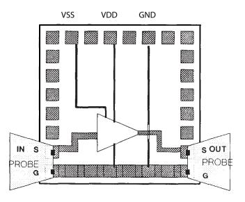
*Figure 4. Typical MMIC padout, ground-signal probes in contact*
