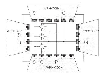
Figure 30. Typical digital IC padout
