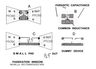
Figure 35. Optimization of small silicon transistor characterization device. Dummy device is used to correct measurement for remaining parallel-capacitive parasitics.
