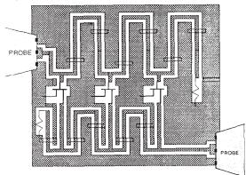
Figure 25. MMIC layout, with padouts for probes.
