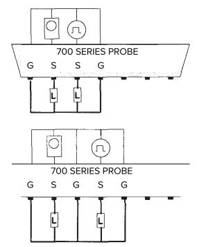
Figure 20. Circuit used to measure crosstalk between S1 and S2 in WPH-700 series multicontact probes. Load L was either an open, short, or 50 ohms.
