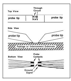
Figure 2. Probe tip: top, bottom, and side view.
