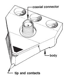
Figure 1. Coplanar probe
