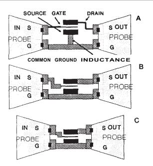
*Figure 33. Optimization of large GaAs FET characterization device*
