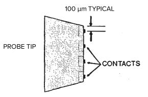
Figure 5. Substrate extension is typically 100  $\mu$ m. probes in contact.
