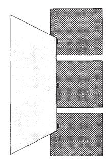
*Figure 38. Off-center probe landing on large hybrid or package pads.*
