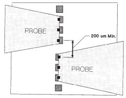
Figure 10. Rule 104. minimum pads spacing with opposing, side-by-side probes is 200  $\mu$ m.
