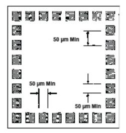
Figure 7. Rules 100 and 102. Minimum pad size is 50 x 50 μm. Minimum pad pitch is 50 μm
