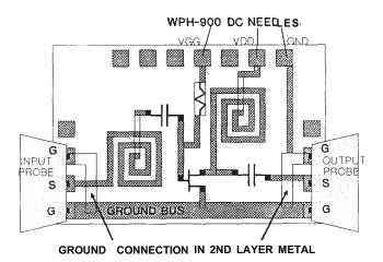
Figure 27. Schematic of lumped-element MMIC. WPH-900 needles provide power, and GSG probes provide measurements. Note short, wide metal used to connect the two ground pads.
