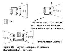
*Figure 36. Layout examples of passive characterization devices*
