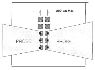
Figure 11. Rule 105. Minimum center-to-center pad spacing for parallel rows of pads with facing probes is 200 µm.
