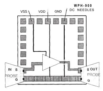
*Figure 23. Typical MMIC with WPH-900 probe needles providing power and ground. The needle inductance can result in circuit malfunction.*
