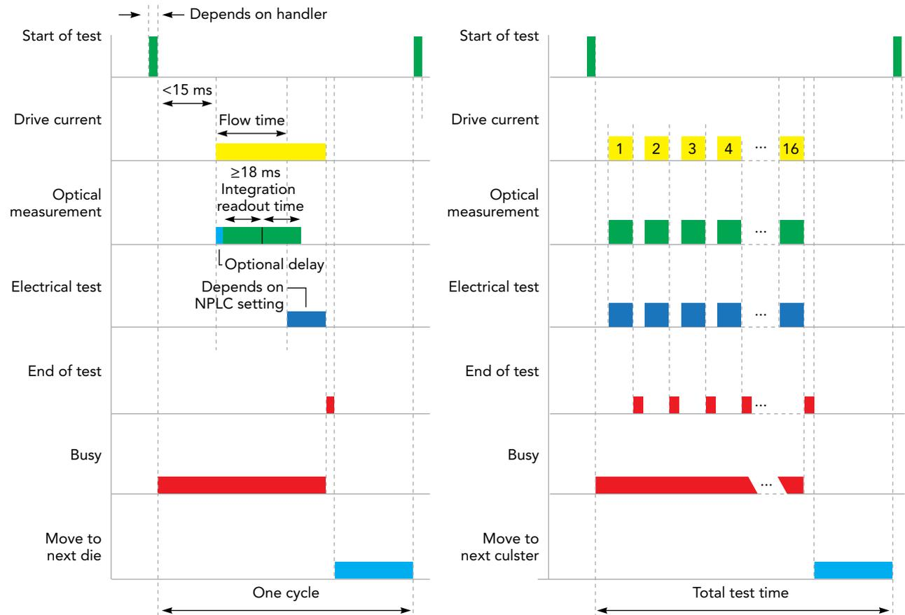
**FIGURE 2.** These timing diagrams for (left) single-die test and (right) multidie test show that a time-consuming move to the next test region is performed after every die for single-die testing, but only once for every 16 dice tested using multidie test.
