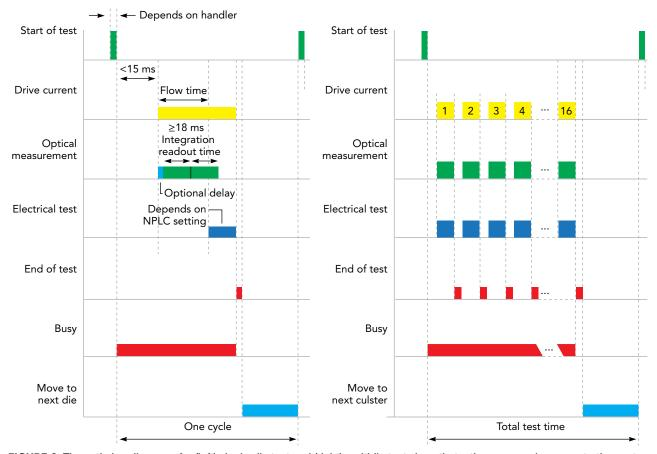
FIGURE 2. These timing diagrams for (left) single-die test and (right) multidie test show that a time-consuming move to the next test region is performed after every die for single-die testing, but only once for every 16 dice tested using multidie test.
