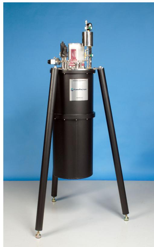
Model HE-3-SSV-PT-2 Cryogen-Free Helium-3 Cryostat
