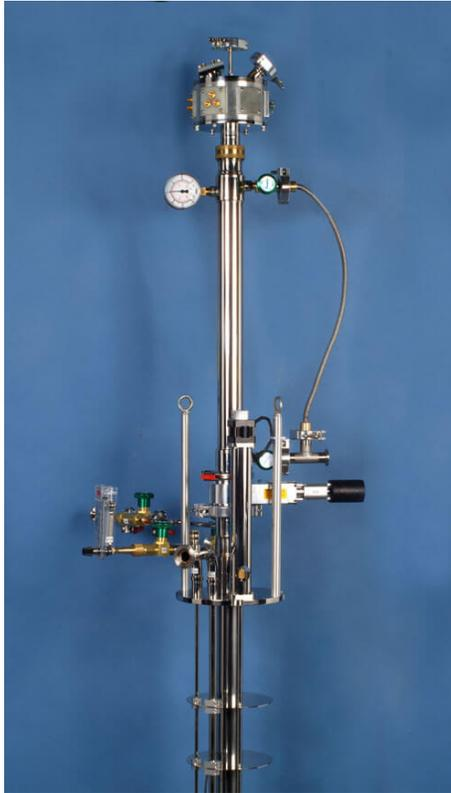
Top View of Model HE-3-TLSL Helium-3 Cryostat
