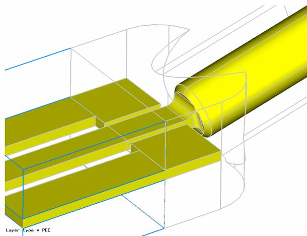
**Fig. 6: Schematic view of the coplanar to coaxial transition**
