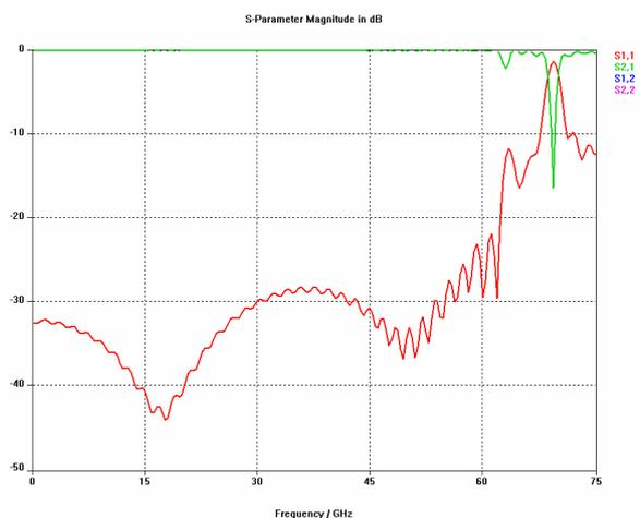
**Fig. 4: Calculated matching of a millimeterwave probetip**
