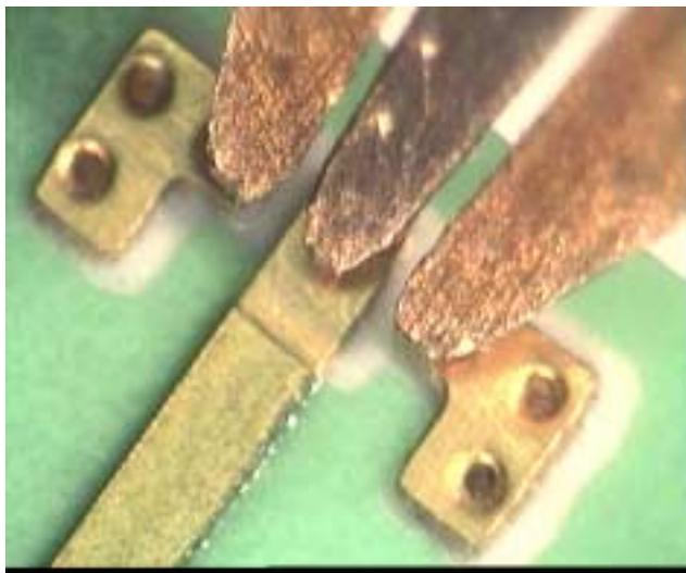
**Fig. 2: Probe tip contacts microstrip line**
