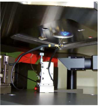
Electrical contact of the DUT from the back side: A back-side camera is located beneath the chuck and views upward in order to position the probes.
