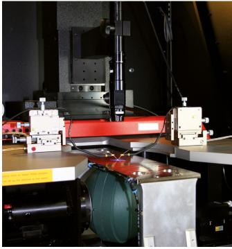
Spectrum analysis of optoelectronic devices with an integrating sphere.  $% \label{eq:control}%$
