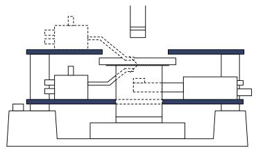
Simultaneous electrical contact of the DUT from the front side and the back side.
