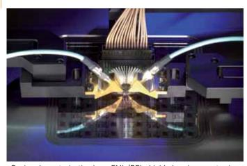
Device characterization in an EMI-/RFI-shielded environment using the  $|\boldsymbol{Z}|$  Probe® and ProbeWedgeTM.
