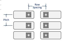
Pitch and spacing of Pyramid Probe card.
