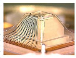
Pyramid Probe membrane features guarded traces to the probe tip. The fixed probe tip placement eliminates manual planarity and alignment adjustments.
