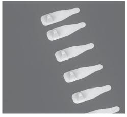
Pyramid Probe tips feature a 12  $\mu$ m x 12  $\mu$ m contact area for probing 30  $\mu$ m x 30  $\mu$ m aluminum and copper pads.
