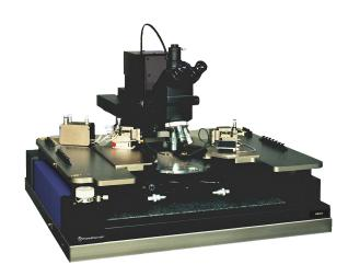
axes of the chuck stage can be moved easily and individually for fast coarse adjustment. Each axis has been designed with an individual magnetic lock and a vacuum brake that enables the fine glide chuck stage to be exactly positioned whenever you release the button. Fine adjustment is ensured for X and Y by high-precision micrometers.
