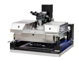
The superior mechanics of the probe system are the basis for stable and precise system setup regardless of your application. The X and Y axes of the chuck stage can be moved easily and individually for fast coarse adjustment. Each axis has been designed with an individual magnetic lock and a vacuum brake that enables the fine glide chuck stage to be exactly positioned
