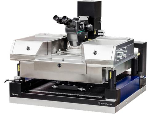
The superior mechanics of the probe system are the basis for stable and precise system setup regardless of your application. The X and Y axes of the chuck stage can be moved easily and individually for fast coarse adjustment. Each axis has been designed with an individual magnetic lock and a vacuum brake that enables the fine glide chuck stage to be exactly positioned whenever you release the button. Fine adjustment is ensured for X and Y by high-precision micrometers.
