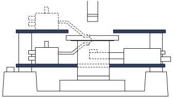
Simultaneous electrical contact and observation of the DUT from the top side and back side.
