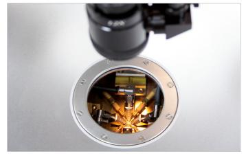
View through the view port of the chamber lid. The shown configuration consists of four RF IZI  ${\rm Probes}^{\circledast}$  and four DC probes.
