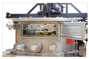
The large front door enables quick and ergonomic loading and unloading of the DUT. The chuck and up to eight vacuum-type positioners can be easily operated from outside of the chamber via universal joint drivers.
