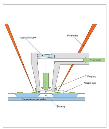
Principle of the Pressure Probe Module. (Patent numbers: DE10000133C2 from 06/26/2003 and DE102005015335A1 from 10/05/2006)
