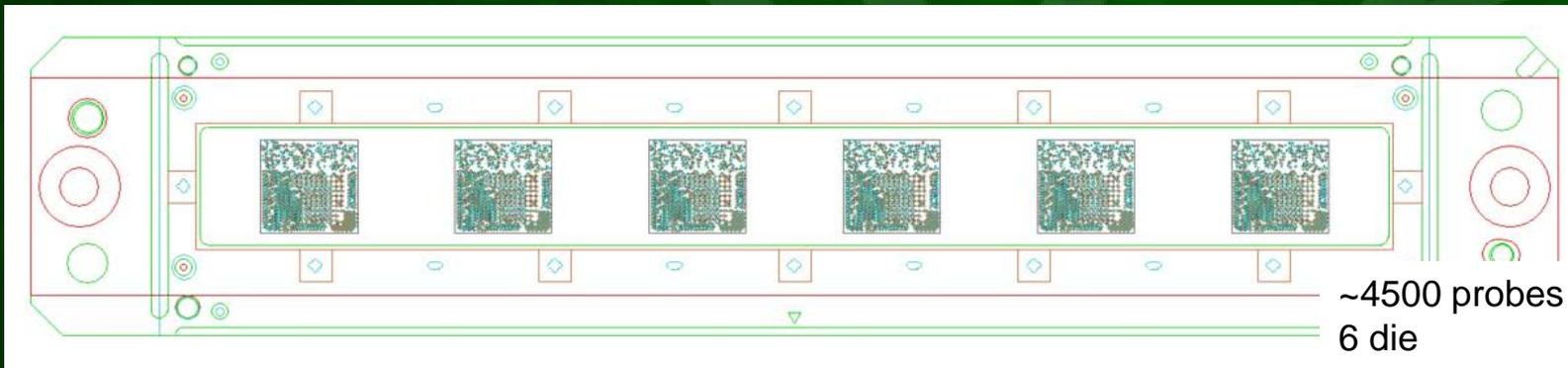
**Vertical MEMS with frequency-capable guide plates can reach down to 106 um grid array pitch. And probe heads are able to support 8+ sites for complex, transceiver-type devices.**
