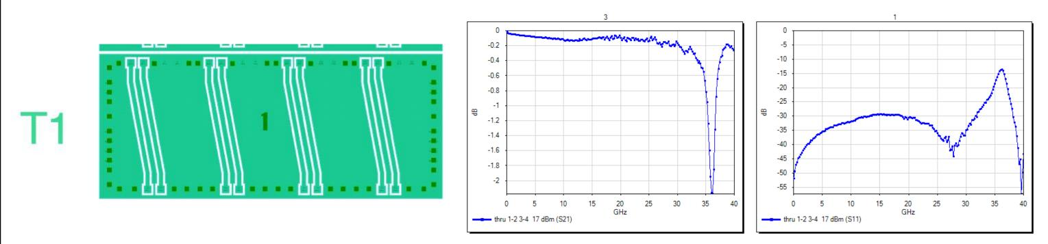
The resonance is occurring withing the pair. Ground in between the pair is not a good ground Not a calibration structure. Good structure to test out
