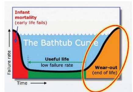
Figure 1. “Bathtub curve” illustrating the realm of intrinsic reliability consideration.
