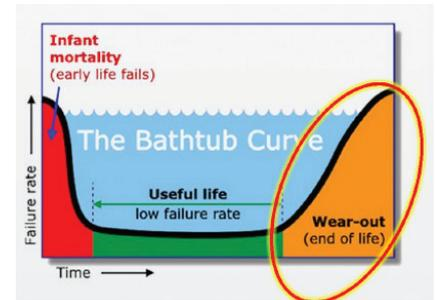
Figure 1. “Bathtub curve” illustrating the realm of intrinsic reliability consideration.
