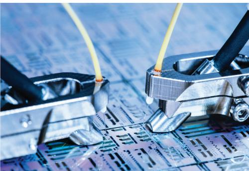
Silicon Photonics wafer-level vertical coupling
