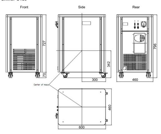
C40s Thermal System: -40°C to +300°C
