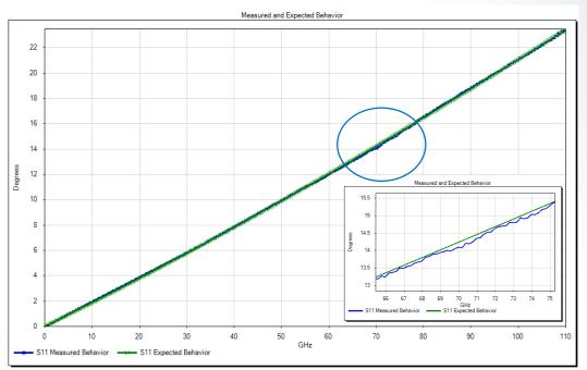
After LRRM calibration, compare the S11 phase of the OPEN to the prediction
