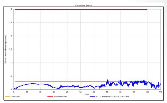
Examine the % difference in the S11 phase measurement of the OPEN
