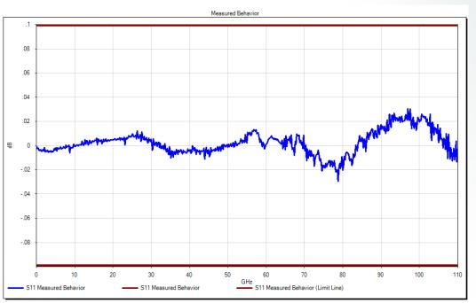
After LRRM calibration, examine S11 of the OPEN treated as unknown by LRRM
