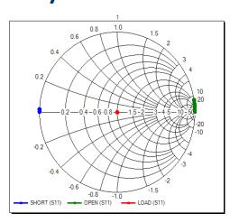
Neither measurement tells much about calibration accuracy, only system repeatability. In many cases the calibration math will drive the solution to equal the calibration coefficients.
