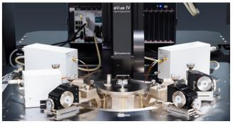
Figure 1: Test setup for chamber noise data using Keysight E4727A (A-LFNA). Three DCP-HTR probes connected to drain, source, gate terminals. All probes inside the probe station MicroChamber shielding environment.
