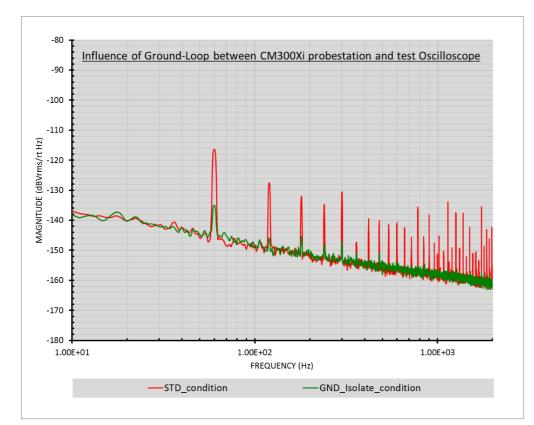
Figure 4: Measurement of chuck noise with Keysight Oscilloscope. The STD condition with groundloop shows more than 30 power line fundamental and harmonics noise spectrums. With the improved GRD isolated condition, the power line fundamental and harmonics noise spectrums are dramatically reduced. (Note: 60 Hz power line spectrum is only -20dB (= 1/10) reduced.)
