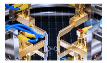
temperature, overcoming the high-temperature performance limitations of standard coaxial needles. The optional probe tips with small diameter are ideal for probing pads as small as  $30 \times 30 \mu m$ .
