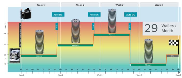
Figure 7: CM300xi-ULN with Wafer Loader MHU301 and Autonomous DC Measurement Assistant achieves 4.1X increased wafer throughput and requires 92% less test engineers time than Figure 5.\*
