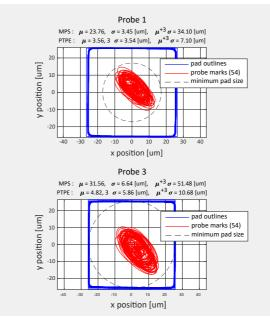
Figure 4: Measured data: 54 sets of die touchdowns / probe scrub marks, at multiple locations across 300 mm wafer, with accurate touchdown of 4 motorized probes on 30 µm pads, at 6 different temperatures ( 25, 150, -45, 175, -55, 200°C). Conditions include wafer soak 3 hr, die soak: 10 min, and 30 min contact test time.
