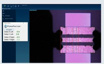
Application example displays probe offset from trained position. Multiple recognition targets allows full analytical freedom.
