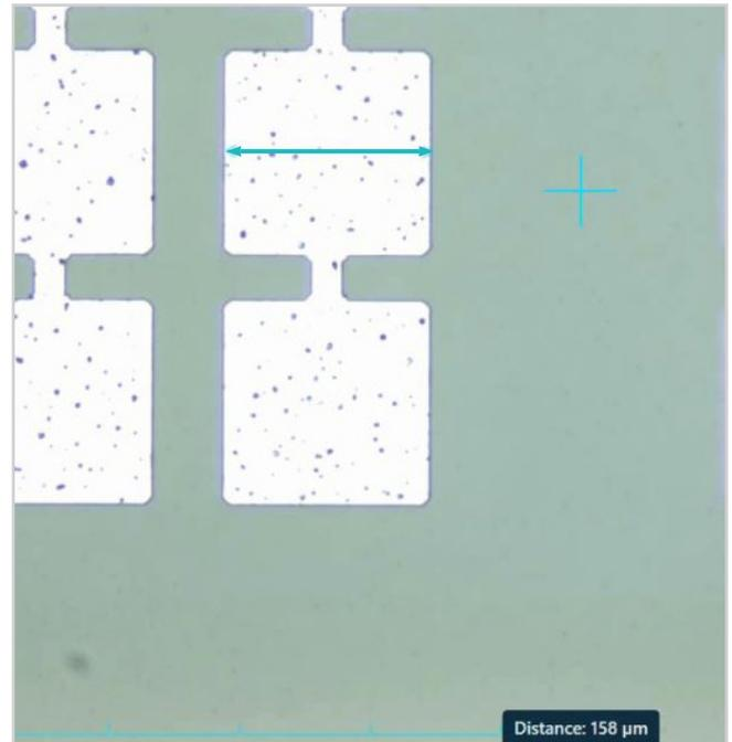
Analytical tools like Measure On-Screen enable comprehensive documentation of the measurement process and assist design debug.
