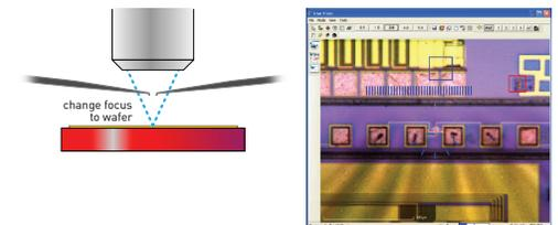
1-4 A corrective move is made to the wafer in X and Y to compensate for position error. The wafer is then moved into the contact position with a correction for the Z error to maintain proper overdrive while the microscope follows the movement of the wafer allowing a focused image of the probe tips and wafer.
