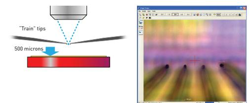
1-3 The microscope is focused on the wafer surface, de-focusing the probe tips, allowing a clear view of the wafer. An autofocus routine finds the Z height of the wafer using the fine focus drive in the microscope. The wafer target location is then found automatically in X and Y using a pattern matching routine.
