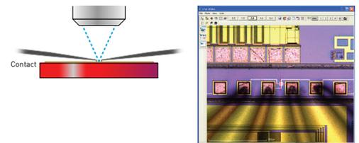
1-2 To train or track the probe tips, the wafer is first lowered in Z to "de-focus" the wafer surface features, allowing a clear representation of the probe tips. This move is only about 2.5 times greater than the "separate" position. During probe tip tracking, the microscope is scanned in Z to find the best match for the probe tip location trained on during the set-up. From this information, the X, Y and Z locations are determined.
