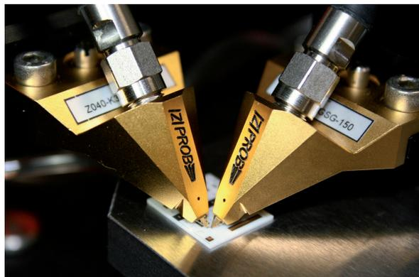
Making HF wafer contact
