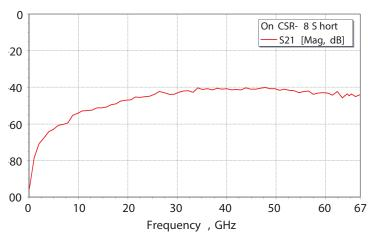
Signal isolation (crosstalk) of two IZI Probes separated by a distance of 150  $\mu m.$
