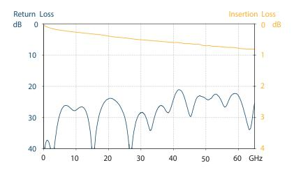
Uncalibrated performance of a |Z| Probe 67 V3N GSG 150.
