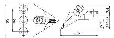
$\left|Z\right|$  Probe standard case (all dimensions in mm).
