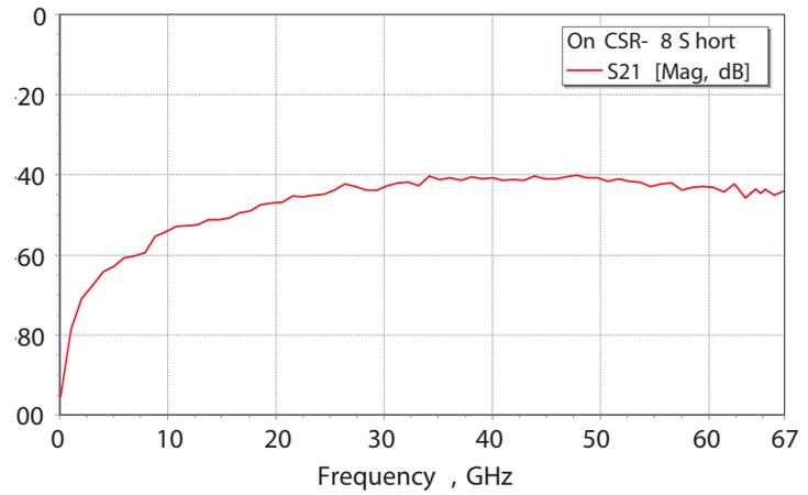
Signal isolation (crosstalk) of two IZI Probes separated by a distance of 150 μm.
